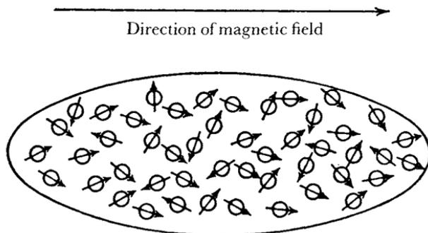
Fig. 1. Paramagnetism.
